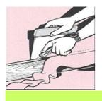
Take the roll, **cut** the wall coverings and the tube at the distance between ceiling and floor + 2" (5cm). The actual cutting line becomes the upper side of the wall coverings. Always use sharp blades ! Put your **glue** onto the wall by means of a **paint roller** in vertical <u>and</u> horizontal direction.
