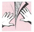
An air pocket may be formed if you do not press or smooth out the wall coverings sufficiently. Cut the air pocket vertically, apply the required adhesive carefully and fit together gently.
