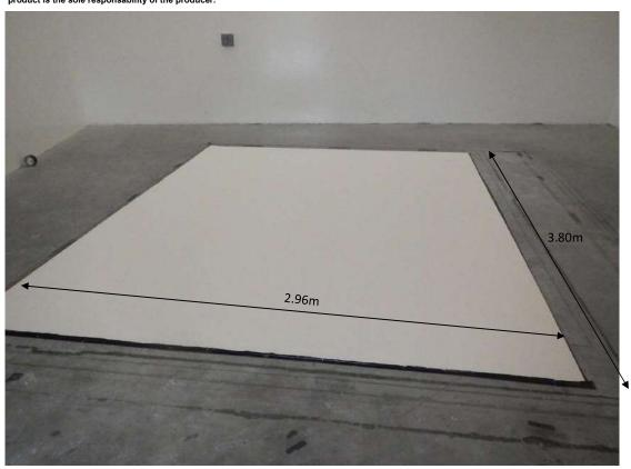
The product is glued on gypsum boards laid directly on the floor surface, according to mounting type B (EN ISO 354:2003 - Annex B). The perimeter of the gypsum boards is tightly butted and sealed to the floor by means of an acoustically reflective tape.
