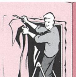
Cut away around windows and doors. Roll out the wall coverings across windows and doors. Then cut away the openings, leaving sufficient material for a neat finish around the frames. Save all left-overs, **do not fold them**, use them for an invisible finish in other places.
