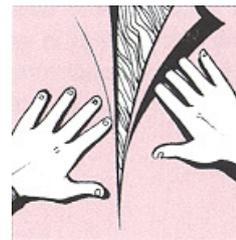
An air pocket may be formed if you do not press or smooth out the wall coverings sufficiently. Cut the air pocket vertically, apply the required adhesive carefully and fit together gently.
