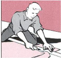
Take the roll, **cut** the wall coverings and the tube at the distance between ceiling and floor + 2" (5cm). The actual cutting line becomes the upper side of the wall coverings. Always use sharp blades ! Put your **glue** onto the wall by means of a **paint roller** in vertical and horizontal direction.
